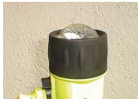
out and discolor. Had something been close by with a low flash point, a fire could have easily started. One doesn't need much imagination to think what the result of that could have been. Also the light was packed with the switch in the locked position! So much for locks on the switches.
